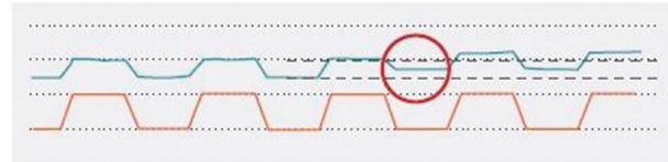
Overall increase in consumption → Anomalia/leakage in supply or upstream of valve
