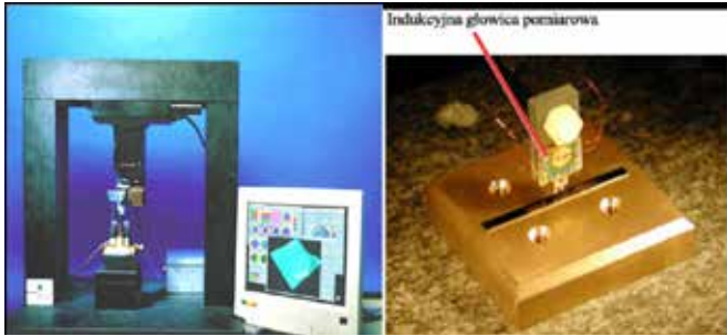
Rys. 22. Stanowisko BEMI – Barkhausen Eddy Current Microscope izfp
