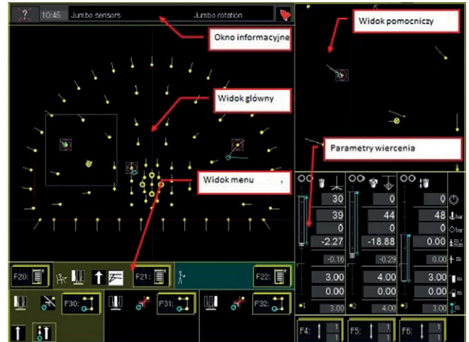
Fig. 5. View of control panel window of BeverDrill system
